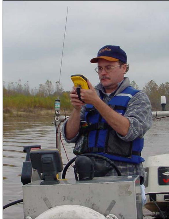
Figure 13 – GPS receiver used for recording positions on the river.
