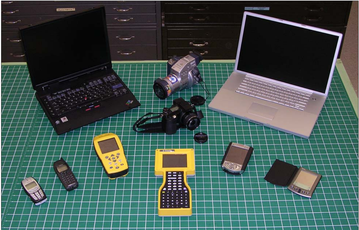
Figure 7 – Modern technology enabled accurate and efficient collection of mapping data in the field. Pictured are the laptop computers, person digital assistants (PDA or “Palm” units), GPS receivers and data recorders, cellular phones, and digital cameras used in the project.
