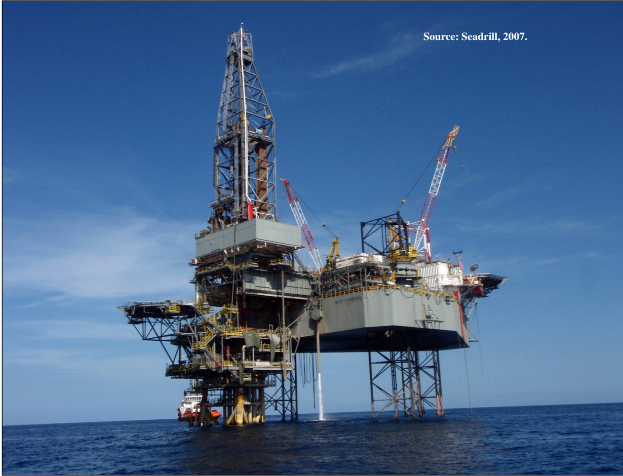
Figure A.15. A cantilevered jackup rig operating at a platform.
