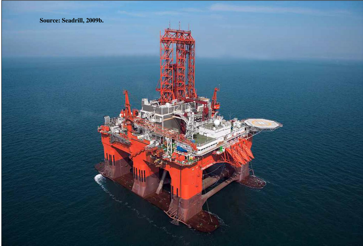
Figure A.21. West Eminence , a 6 th generation semisubmersible, built in 2009.
