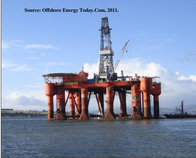
Figure A.19. Essar Wildcat , a 2 nd generation Aker H-3 semisubmersible, built in 1977.
