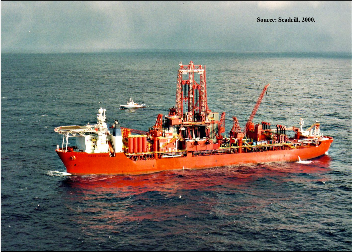
Figure A.24. A modern drillship, the 5 th generation West Navigator , built in 2000.
