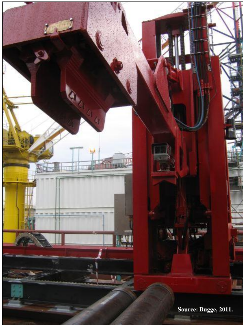
Figure J.14. Pipe deck machine.
