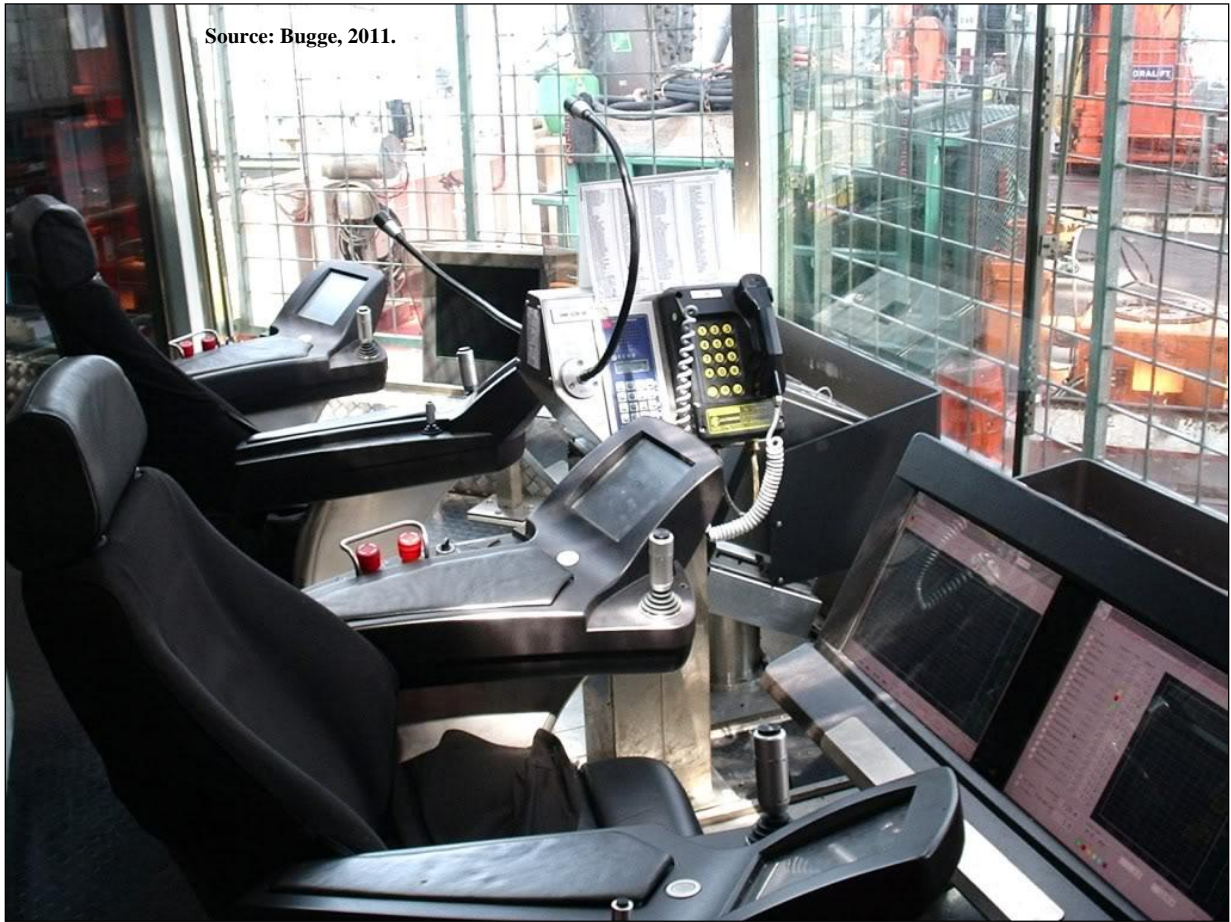
Figure J.15. Drilling control stations.
