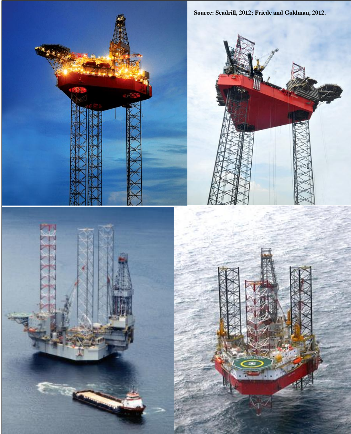
Figure H.14. Commonly built international jackups; clockwise from upper left: KFELS B Class, Gusto MSC CJ70, Pacific Class 375, F&G JU 2000E.
