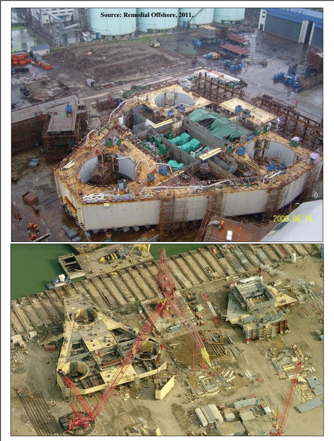
Figure I.4. Hull construction of a F&G Super M2 rig (top) and two LeTourneau Super 116s at the AmFELS Brownsville, Texas yard.
