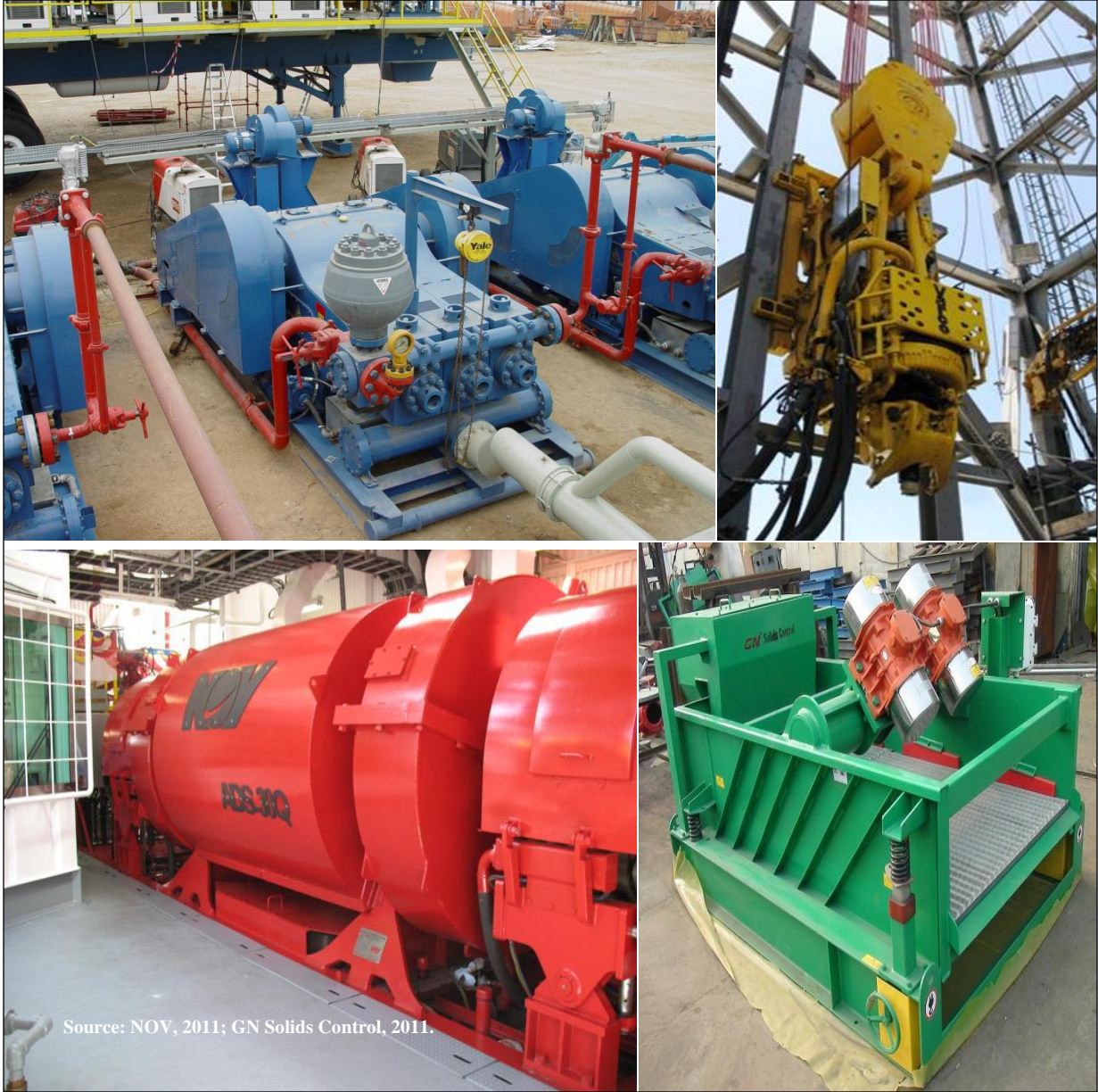
Figure L.1. Drilling equipment; clockwise from upper left; mud pumps, top drive, shale shaker, drawworks.
