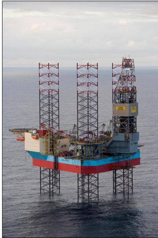
Figure H.6. Cylindrical and trussed legs on the Bethlehem MS-225 Spartan 202 and Gusto MSC CJ70 Maersk Inspirer .
