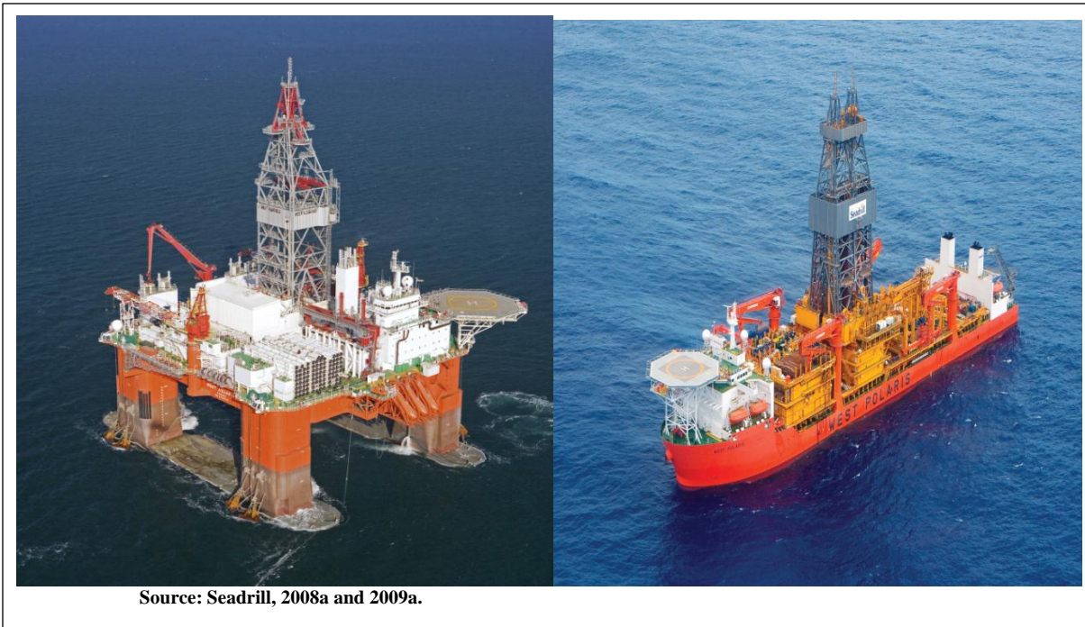
Figure A.8. Floating rigs. Left, the West Aquarius , a semisubmersible; right, the West Polaris drillship.
