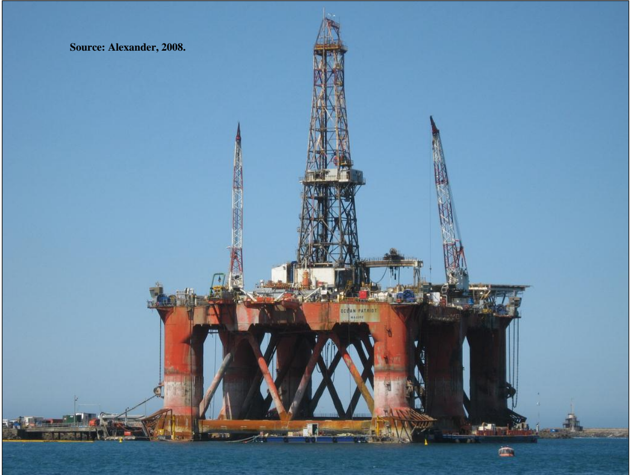
Figure A.20. Ocean Patriot , a 3 rd generation Bingo 3000 semisubmersible, built in 1983.
