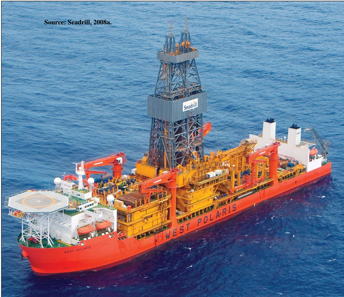
Figure A.25. Dual activity derrick on the 6 th generation West Polaris drillship built in 2008.
