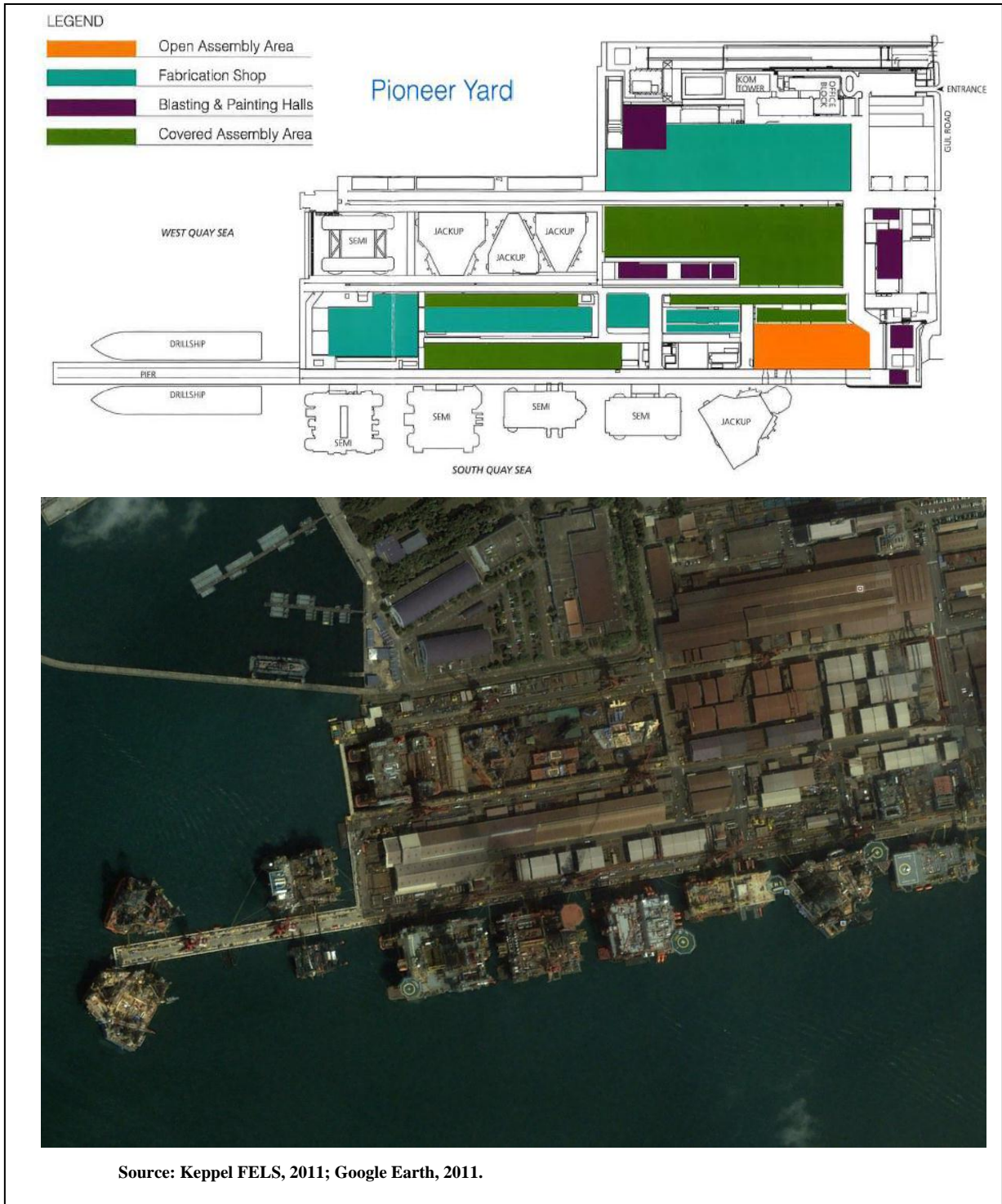
Figure G.6. Layout of the Keppel FELs shipyard in Singapore and satellite view in 2011.
