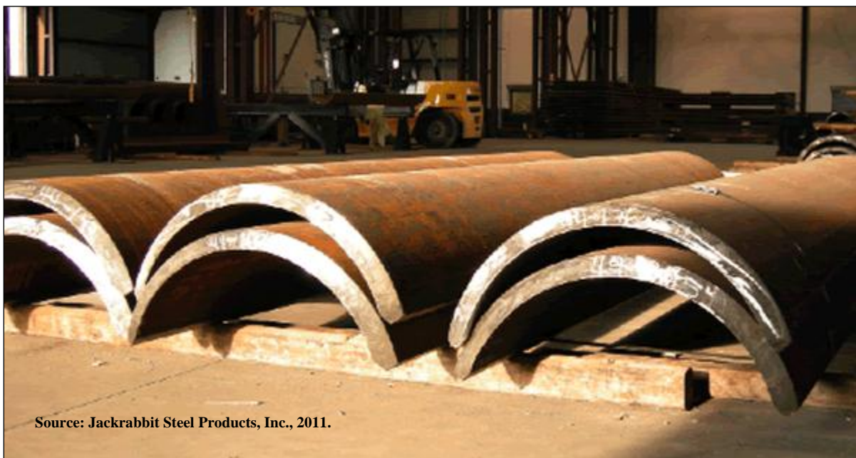
Figure I.7. Formed half chords pressed by Jackrabbit Steel.
