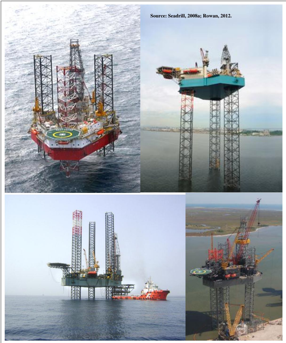
Figure H.2. Four common rig designs; clockwise from upper left: BMC Pacific 375; KFELS N class; LeTourneau 240 C; LeTourneau Super 116E.
