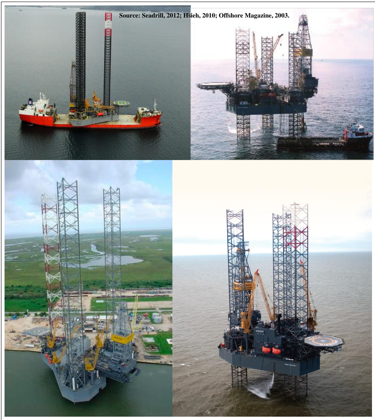
Figure H.11. Common U.S. built jackup designs; clockwise from top left: LeTourneau Super 116E, LeTourneau Tarzan, LeTourneau 240C, LeTourneau Super Gorilla XL.
